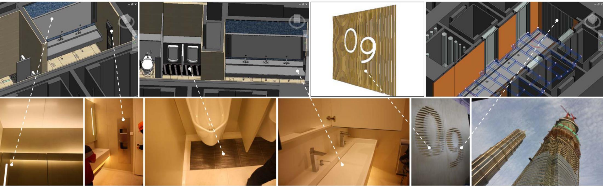
BIM Model vs. On-site Installation Results
