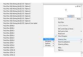
4. Import/Link Geometry: Once geometry has been exported it will need to be brought into 3ds max. It is important files be linked and NOT imported. Quick animations should be used to help aid the design process and therefore will be constantly changing and being updated. If you have been diligent with material application while building your geometry then you can import "via material from Revit". If you have been lax you might want
