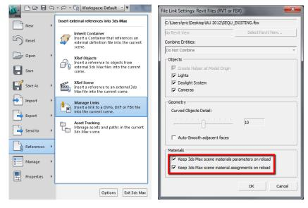
to import via individual elements so that you can apply materials more precisely to individual geometry objects. When geometry is linked insure that the "keep materials on reload" option is checked.
