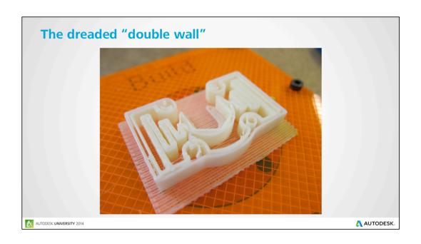
Double walls appear when the wall thickness is not an even multiple of the layer width. The slicer doesn't know what to do with the missing area.
