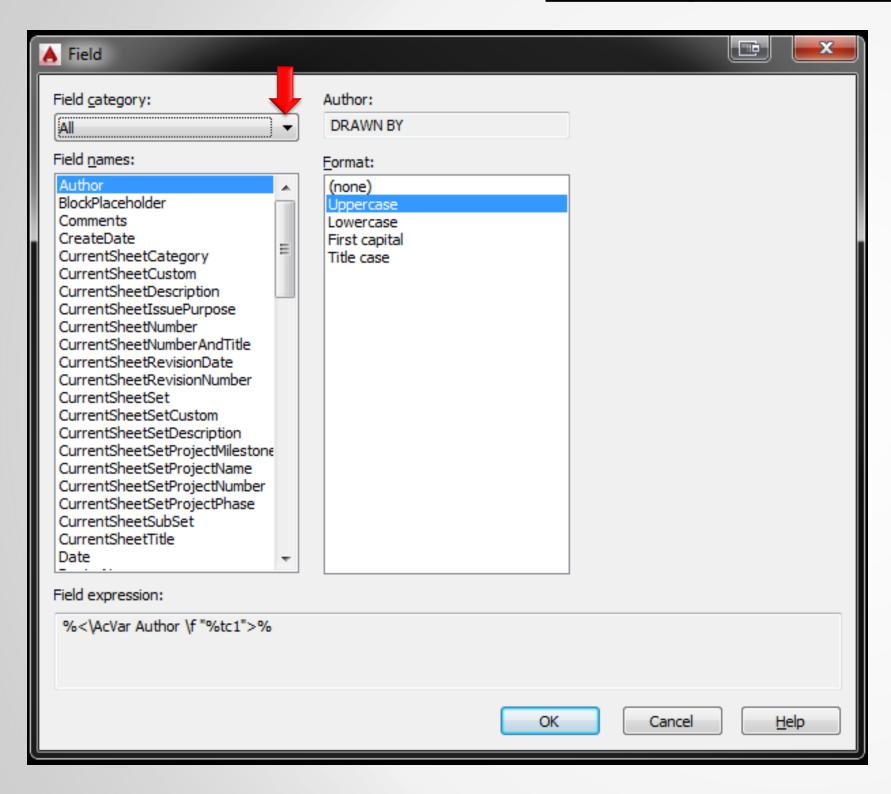
AutoCAD Fields are information (data) that is stored within the DWG file or from an external data file (like SSM's dst files) These fields are very versatile and are able to be edited with ease. Editing one will change all instances of that field (similar to blocks), but can be used across multiple DWG files.
