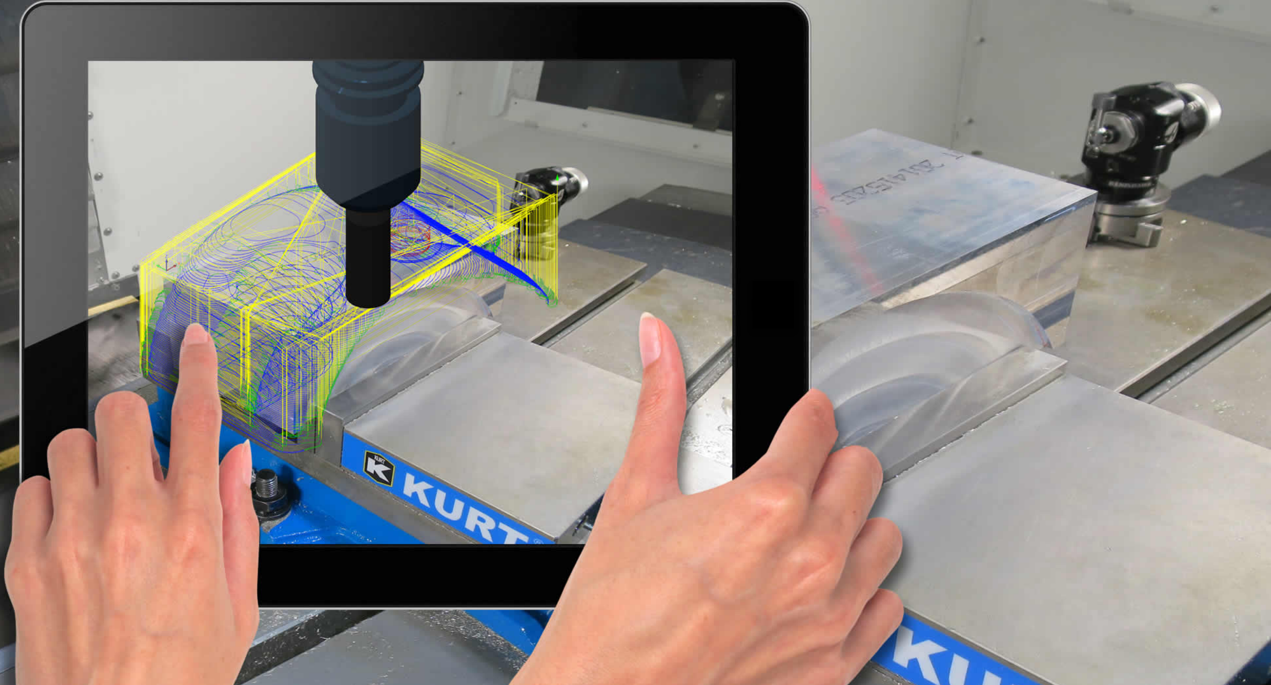
Augmented Reality Prototype: Fusion 360 CAM toolpath data overlaid on CNC
