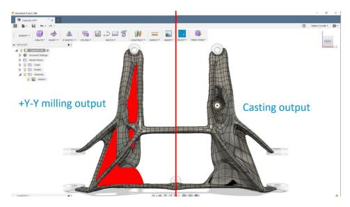
I can define as well the parting plane for the mold and removing the undercuts. Find the detailed steps in <u>this video</u>
