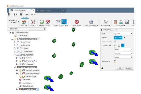
After having defined the Load Cases, I specify the objectives for our results, that, as I wrote above, is mainly to reduce the mass of the existing design and I set a Safety Factor of 5.
