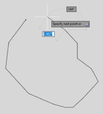
Specify next point or [Arc/Close/Halfwidth/Length/Undo/Width]: Specify next point or [Arc/Close/Halfwidth/Length/Undo/Width]:
