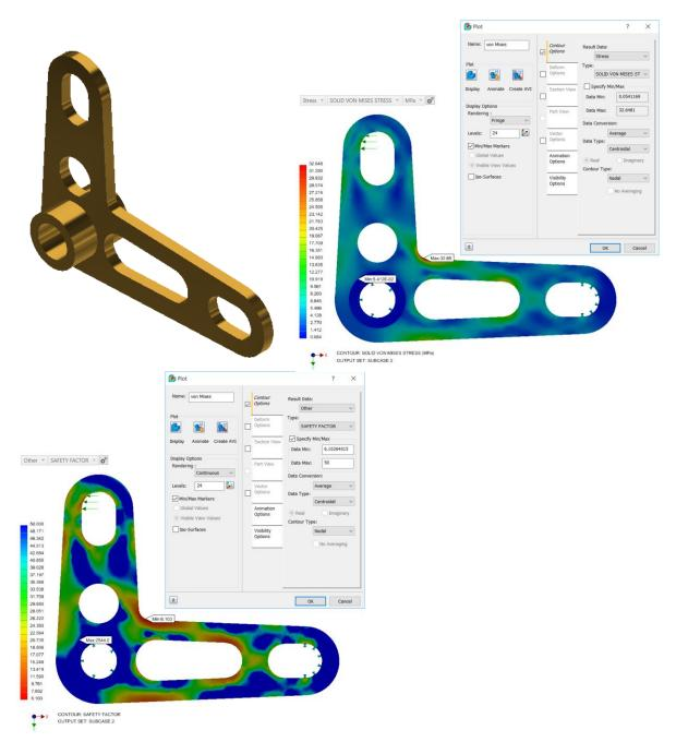
Inventor Nastran Safety Factor plot value of 6.103 is the same as the calculate value of 6.12, based on the average centroidal stress result.
