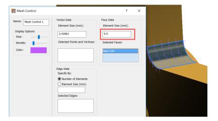
19. Click OK > Select Mesh Settings > Specify 1 for Element Size (mm) > Select Settings to access Advanced Mesh Settings > Specify 1.1 for Max Element Growth Rate.
