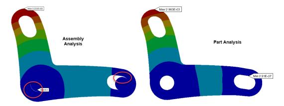
We can see that the assembly analysis shows more movement which is due to the separation contacts allowing the lever to separate from pins, like reality. This behaviour cannot be simulated in part analysis. The extra movement in the assembly will result in a higher stress than the part analysis.
