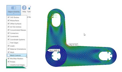
The maximum von Mises stress has now increased to 9.726N which is about 5% increase in value. The percentage change in maximum von Mises stress value has reduced and suggests the max value will eventually converge by further mesh refinement. At this stage we can take this value to calculate of our safety factor or we can alternatively run one more simulation with a finer local mesh. We will use the latter option.
