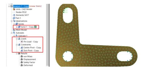
An alternative method is to create a new analysis and then drag and drop boundary conditions and other settings from the model tree to the analysis tree.
