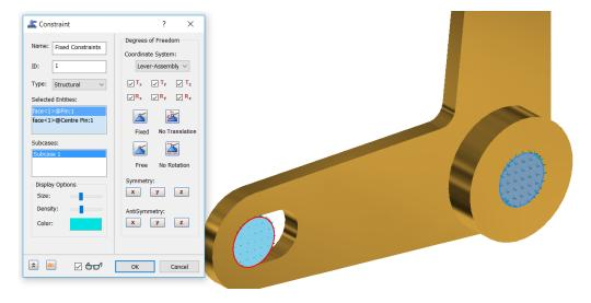
5. Select Frictionless Constraints > Select all 3 highlighted faces to apply new constraint > Specify Z-Symmetry for Name > Select Preview so you adjust display options as desired
