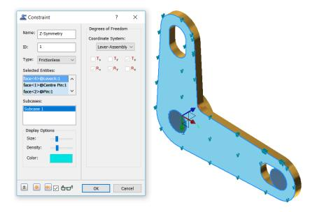
6. Click OK > Select Loads > Specify Pin-Load for Name > Select Bearing Load for Load Type > Select Components for Direction > Specify -15 for Magnitude in Fx field > Select Preview so you can adjust display options as desired.
