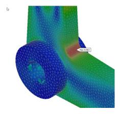
The maximum von Mises stress has increased to 9.903N which is about 1.8% increase in value from the 3<sup>rd</sup> analysis results. So, we can confidentially say the results have converged. We have a safety factor value of 20.
