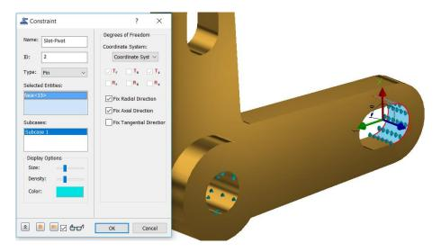
8. Click OK > Select Loads > Specify Pin-Load for Name > Select Bearing Load for Load Type > Select Components for Direction > Select highlighted cylindrical face to apply constraint > Specify -30 for Magnitude (N) in Fx field > Select Preview so you can adjust display options as desired.
