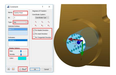
Applying a pin constraint will automatically create a customised cylindrical coordinate system with reference to the selected cylindrical face.
