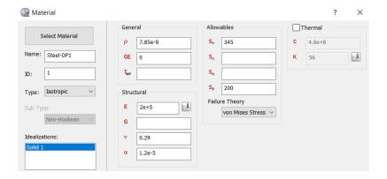
You can see the G field is blanked out. Here you can amend or add further values as required. Any additional data defined here will be saved only within the part file.
