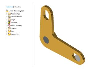
Extrusion 1 is defined in the assembly environment as it is easier to half all parts in one extrusion when compared to extruding in part environment for each component. The other advantage of this method is it does not alter the original parts.
