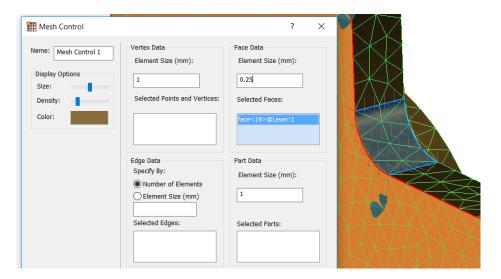
**8.** Click **OK** > Select **Mesh Settings** > Specify **1** for Element Size (mm) > Select **Settings** to access Advanced Mesh Settings > Specify **1.1** for Max Element Growth Rate > **Click OK**.
