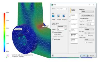
This is very close to the Safety Factor plot value of 21.07 with a difference of less than 0.5%.
