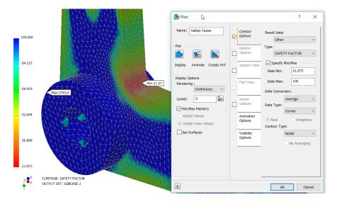
The minimum safety factor, in same location, is 21.07 slightly higher than the previously calculated value. So, the question is why are the values different? The answer is that the calculated stress value is based on the average stress value at the node location. Whereas the safety factor plot values are based on taking the average of the nodal safety factors. This can be best explained by the following example. We will use 200MPa for yield limit for comparison purposes.
