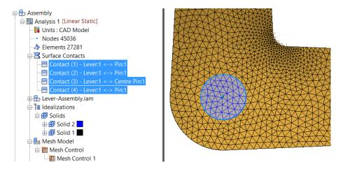
This will create 4 bonded contacts between lever and the two pins. Pins in reality, are not bonded and instead allow rotation and possible separation from the lever when a high enough load is applied.
