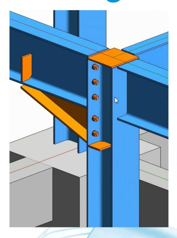
Steel Connection Detailing
