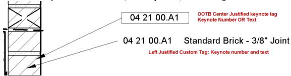
The OOTB detail item tag references the Type Mark value is center justified, and can be boxed or not. Utilizing a value other than Type Mark might be beneficial to gain more flexibility while tagging. For instance, a tag can use the Type Comments and/or Comments to allow for consistency in the Type Comments, but to also allow for flexibility with individual notes by using the instance based comments. A tag can then be set up to allow a user to change the tag type out if desired.
