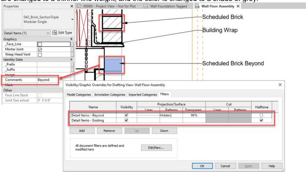
Using filters can eliminate the need for additional family types as well as the manual labor of Overriding graphic in view by Element. Filters also add consistency to a project
