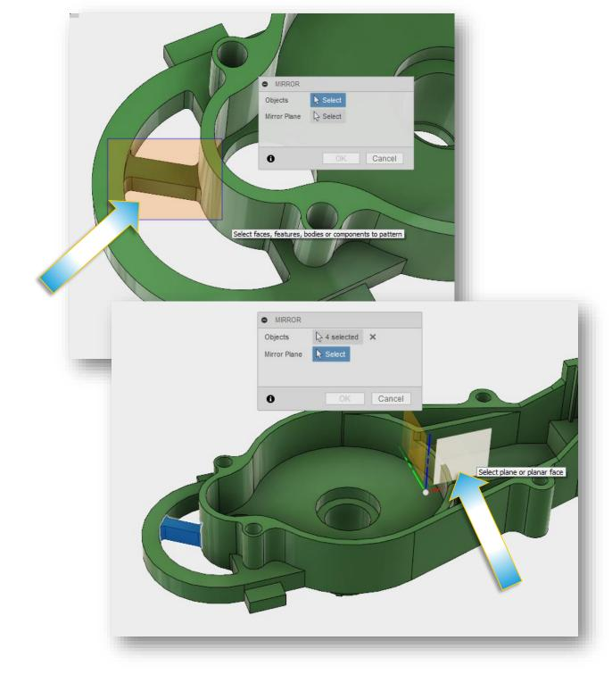
Notice we were able to re-use existing geometry to create a new rib without having to create a sketch or machine away old geometry to create new geometry
