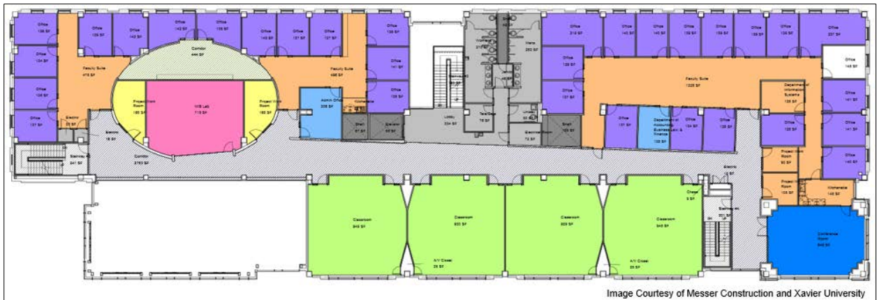
Figure 5– Floor plan in a BIM FM Model without annotation but with space definition.
