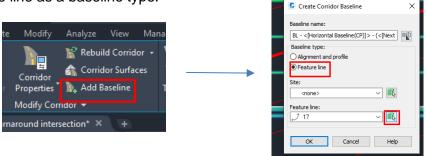
In the "Apply Feature line names" press on the Name Template icon. Just press the "OK" button in the Name Template window and then, press the "OK" button in all previous windows.
