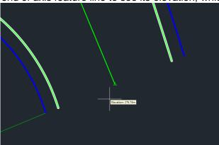
Move the cursour to the end of the radial feature line and adjust its elevation from 0 to 276.74 by left-clicking with the mouse button and typing "276.74".
