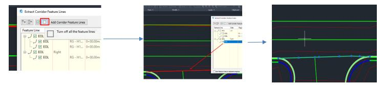
Repeat these steps to create a feature line from the below region. In the "Extract Corridor Feature line" turn off all feature lines and select the first EOL in the list.
