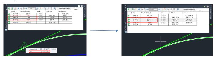
Select the first, second, and third vertexes. Press the "Flatten grade or elevations" command icon. Select the "Constant grade" option.
