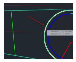
9. Select the corridor=>Ribbon=>Add regions=>Select the first radial feature line=>Right-click with the mouse button=>Fill=>Select Radial\_Lane\_Sidewalk assembly.
