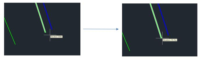
10. Now, we need to deal with two vertexes near the second axis feature line. And we also are going to use the "Quick elevation edit" command.
