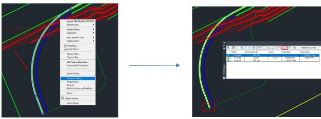
Select the third vertex and check the elevation of the "Top" surface near it. It is supposed to be 276.74/ If it is not – fix it. After that, select all the vertexes and use the "Flatten" command with the "Constant grade" option to fix the second vertex elevation.
