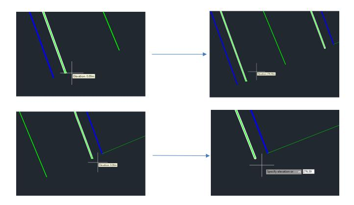
11. Select the first radial feature line, then right-click with the mouse button and select the "Elevation editor" command.
