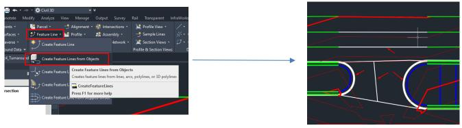
In the "Create feature line" window press the "OK" button. In the "assign elevation" window select the "Top" surface, then press the "OK" button.
