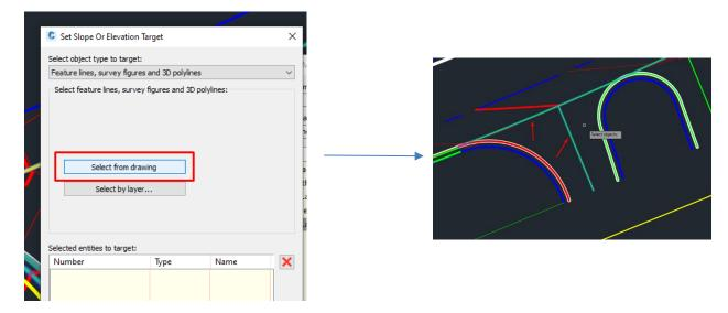
Selected feature lines will appear as Selected entities to target. Press the "OK" button in all windows. You should see our "Top" surface spreading in the new corridor region with nice and smooth horizontals.
