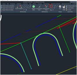
7. Take your cursor near the end of the axis (the begining of the axis is near the corridor) and left-click with the mouse button.
