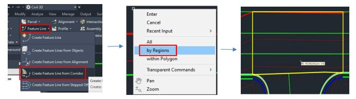
Turn off all the feature lines=>Turn on the last EOL. EOL feature line is done.
