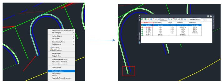
Select the third and fourth vertexes. Then check the appropriate elevations of the "Top" surface near them by leaving the cursor on the main driveway. Input this elevation, which is 276.93, in the elevation column for our vertexes.
