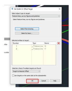
Now, click on "None" for the LaneElevation line, select feature lines as the object type.
