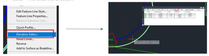
For the first vertex adjust the elevation to 276.73, and for the last vertex 276.86 since these are the elevation of the "Top" surface.
