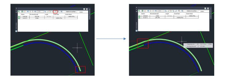
Then, move your cursor at the driveway just a little bit aside from our radial feature line and check the elevation of the "Top" surface. It is 277.11. Input this value for our vertex in the elevation editor.
