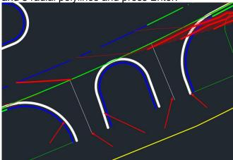
In the "Create feature lines" window press the "OK" button. In the "Assign Elevations" window select the "Top" surface and press the "OK" button.
