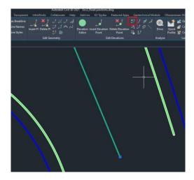
Move the cursor the end of axis feature line to see its elevation, which is 276.74.
