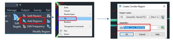
Select three feature lines (turnaround axis and two EOL) as targets for the LaneOffset.
