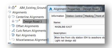
Assign the desired design criteria and design criteria file to both horizontal and vertical. Assigning design criteria assures that when adjustments are made to the horizontal and vertical path violations will be instantly reported and can be remedied instantly.
