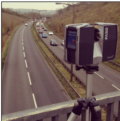
FIGURE 5: PHASE BASED SCANNER CAPTURING POINT CLOUD DATA
