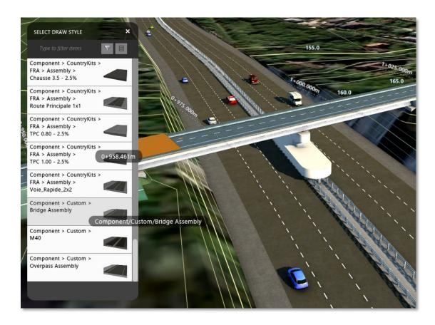
12. Then, using the grips, stretch out the orange/blue rectangle to cover the extent of where you feel the handrailing would start and finish, then press **Return**.
