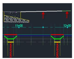
More elaborate subassemblies can be developed to utilize conditional subassemblies. Attaching multiple corridor baselines will display assemblies in cross sections. Add the sidewalk alignment to the corridor and apply this assembly that turns off the walk at driveways and or intersections. Notice the yellow polyline above.
