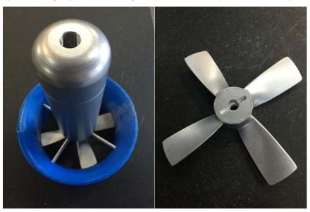
FIGURE 1: THIS AUTONOMOUS UNDERWATER VEHICLE PROPULSION ASSEMBLY DESIGNED AND MANUFACTURED BY RAUCH ENGINEERING USES A CNC MACHINED PROPELLER AND MOTOR HOUSING IN COMBINATION WITH 3D PRINTED COWLING.
