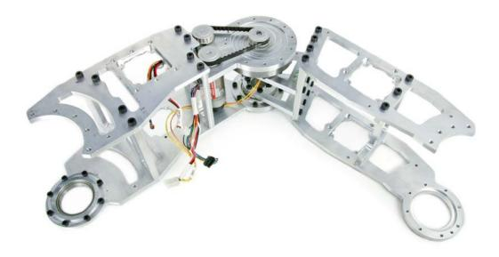
FIGURE 2: RESEARCHERS AT DREXEL AUTONOMOUS SYSTEMS LABORATORY (DASL) USE A PCNC 1100 TO MACHINE STRUCTURAL COMPONENTS SUCH AS THIS LEG ASSEMBLY FOR THE HUBO+ AUTONOMOUS HUMANOID.
