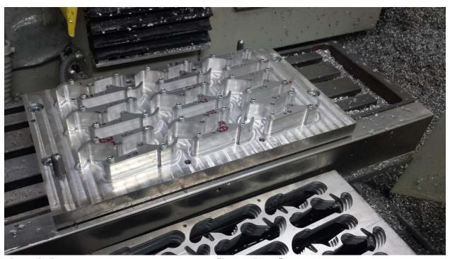
FIGURE 9: THESE PARTS ARE MACHINED BY FIRST USING A "PICTURE FRAME" WORKHOLDING TECHNIQUE TO ROUGH MILL THE PERIMETER PROFILE BEFORE A SECOND FINISHING MILLING OPERATION ON A FIXTURE PLATE.
