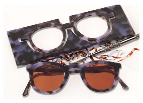
FIGURE 6: INDIVIDJUAL EYEWARE USES A TORMACH PCNC 770 TO CREATE PERSONALIZED SUNGLASSES FOR HARD-TO-FIT CUSTOMERS.
