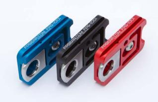
FIGURE 8: THE LONG PARALLEL EDGES OF THIS CAMERA ADAPTOR IS A NATURAL FIT FOR A "FLIP AND DECK" WORKHOLDING STRATEGY USING A MACHINIST VICE.
