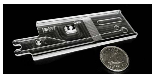
FIGURE 3: A MICROFLUIDIC DEVICE MACHINED ON TORMACH PCNC 770. PHOTO CREDIT: EDMOND YOUNG, UNIVERSITY OF TORONTO
