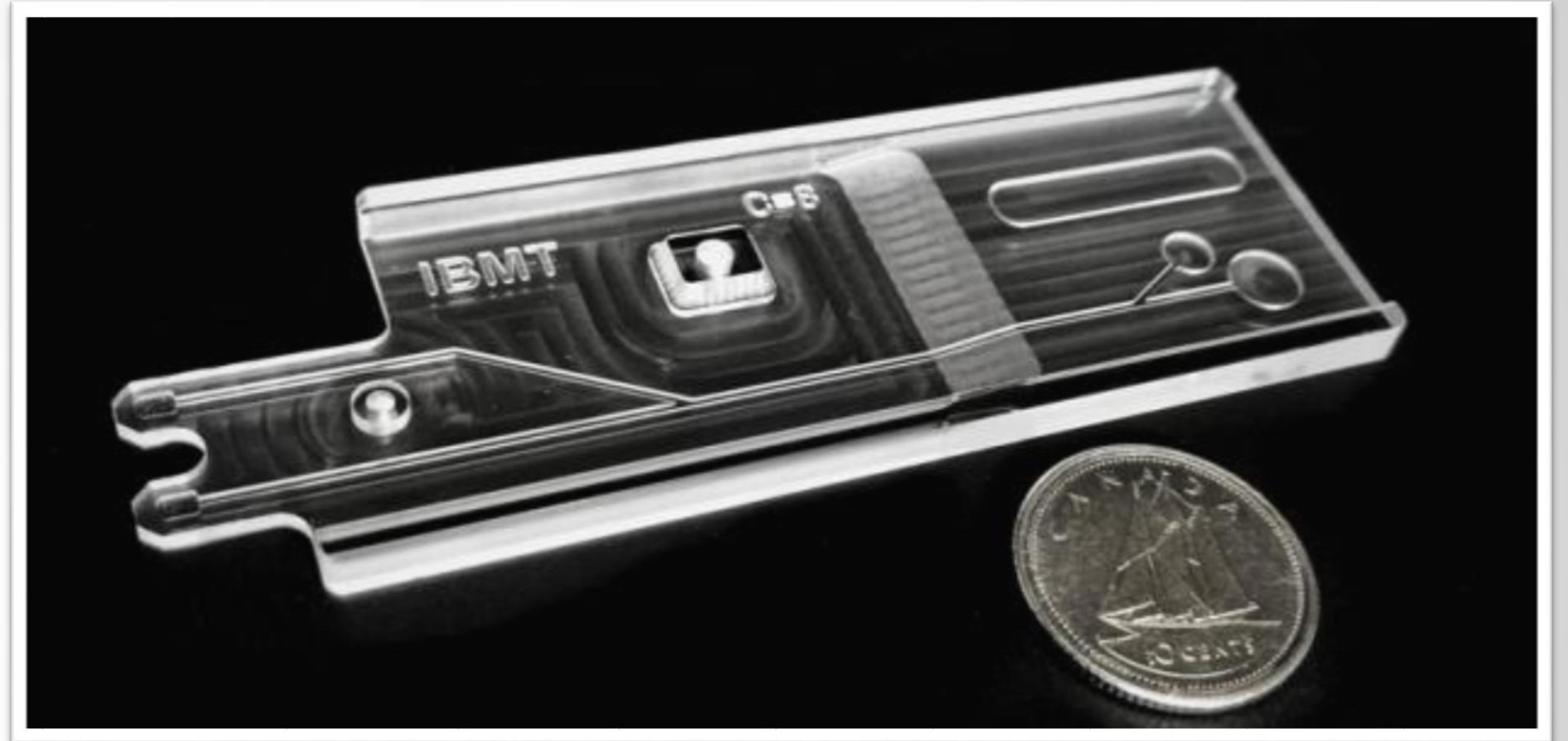
MICROFLUIDIC DEVICE MACHINED FROM ACRYLIC PLASTIC ON TORMACH PCNC 770®. PHOTO CREDIT: EDMOND YOUNG, UNIVERSITY OF TORONTO
