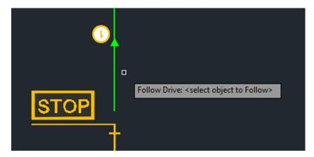
Once the path has been selected you will then set the path properties to be applied to the aircraft. It is here where you can set the point on the aircraft which will track along the line. If you wish your path to be editable once it is in the drawing then you must select the "Create an Editable Path". It is recommended to set the Target Point spacing to no less than 10m, possibly larger for large vehicles.
