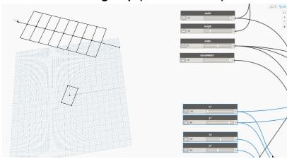
This is a representation in which the parking stalls are mirrored based on the path of the strip. A similar analysis than in the single sided parking strip is calculated to offset the parking stalls from the centerline of the path in the double sided parking strip.
