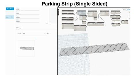
The parking strip has as a base the consecutive single parking stalls that follow a path with a direction and rotation. To calculate the separation of the stalls based on their rotation width and length we have followed this geometry analysis.
