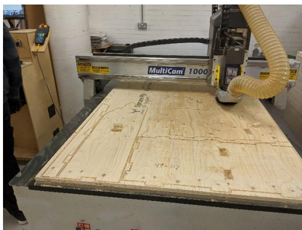
FIGURE 20: OFF-SITE MANUFACTURE OF PROPRIETARY MODULES FOR BESPOKE HOUSING (IMAGES COURTESY OF FACIT HOMES LTD)
