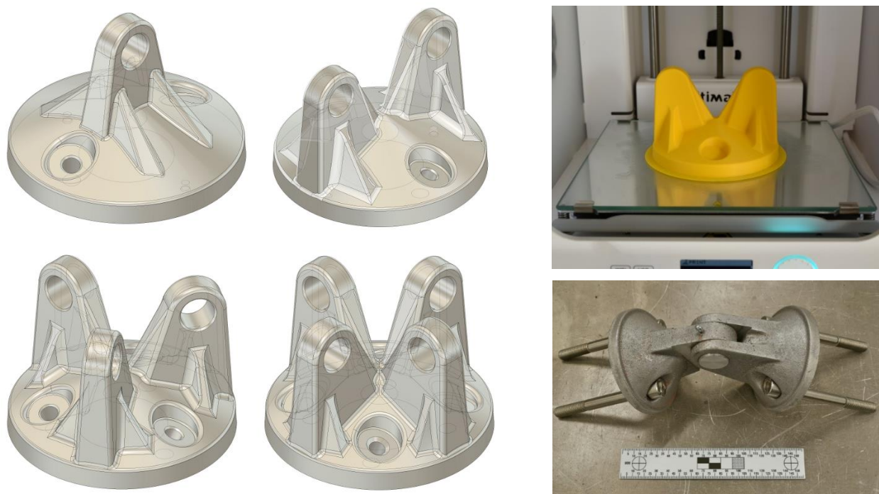
FIGURE 7: 3D PRINTED PATTERNS FINISHED CONNECTOR NODE CASTINGS AND PARAMETRIC VARIATIONS (CASTINGS MADE BY MELIS VAN DEN BERG)
