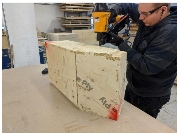
FIGURE 20: OFF-SITE MANUFACTURE OF PROPRIETARY MODULES FOR BESPOKE HOUSING (IMAGES COURTESY OF FACIT HOMES LTD)
