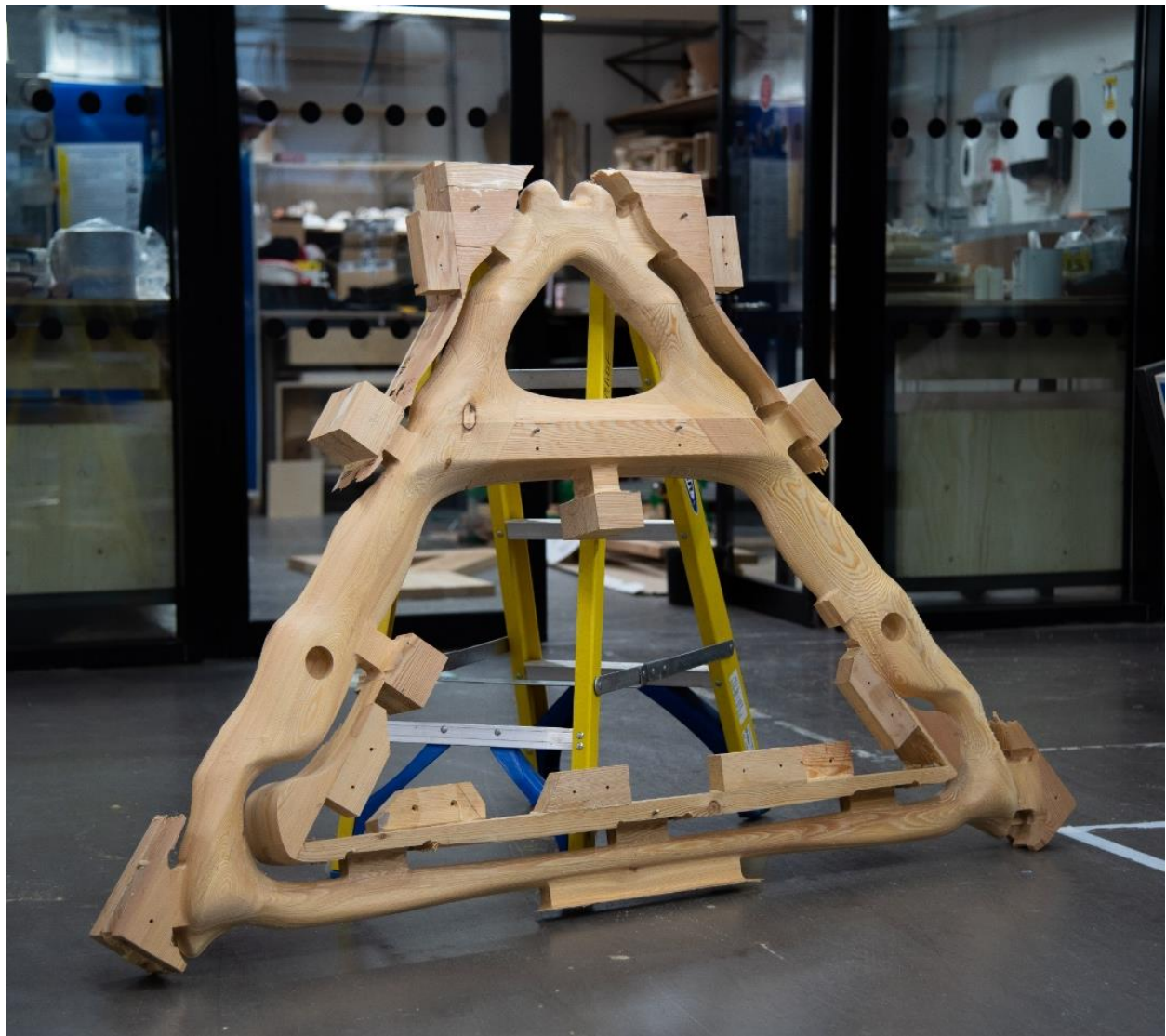
FIGURE 17: STRUCTURAL FRAME SUB-ASSEMBLY 3D CNC MILLED GLUE-LAMINATED TIMBER (IMAGE COURTESY OF WILLIAM-VICTOR CAMILLERI)
