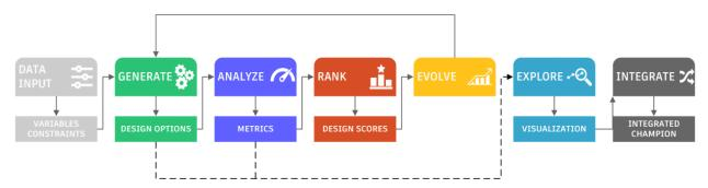
Generative design allows for a more integrated workflow between human and computer, and as a result both are required to undertake a series of steps that allow the process to take place. These steps can be categorized into the following stages: generate, analyze, rank, evolve, explore, integrate.
