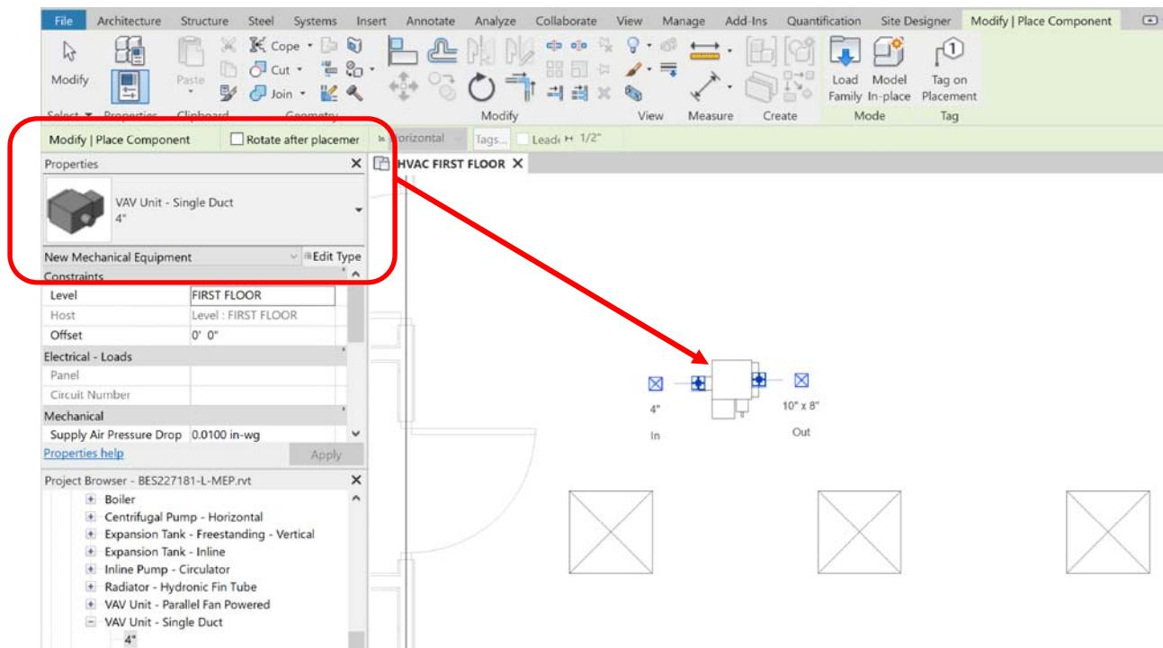
6. Click **Modify** to complete placement of the equipment. Next, to edit the system and add the equipment, **place your mouse over one of the previous air terminals, and then tap the TAB key**. The current duct system will be highlighted:
