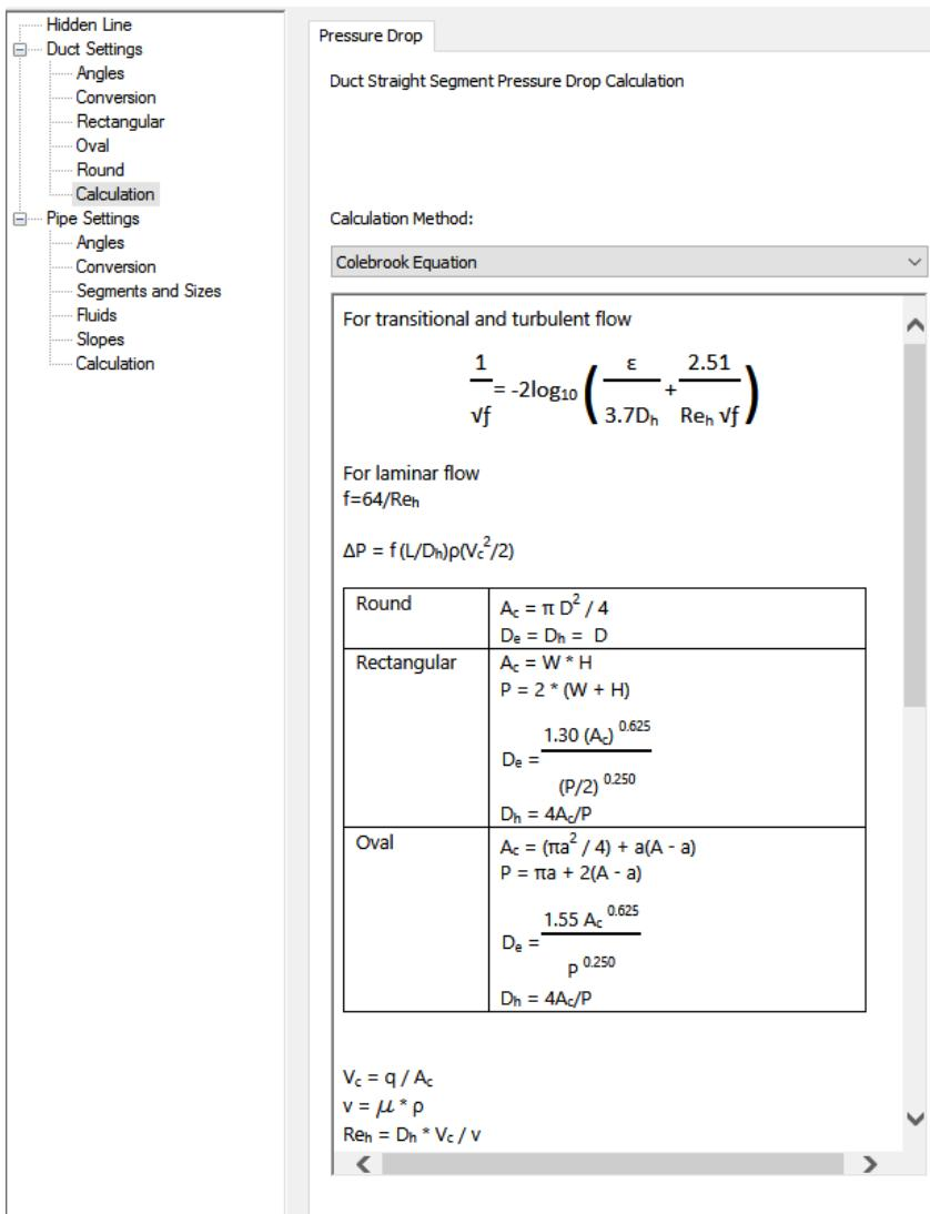
For Calculation Method, select the **Colebrook Equation** pressure drop calculation.
