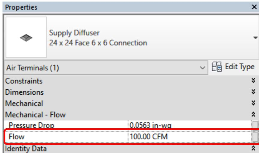
The system is now ready for sizing, and the connected duct will track the air flow values.
