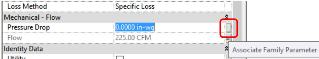
4. The **Associate Family Parameter** dialog appears. You can select **Supply Air Pressure Drop** from the available parameters, which match the formatting of the data:
