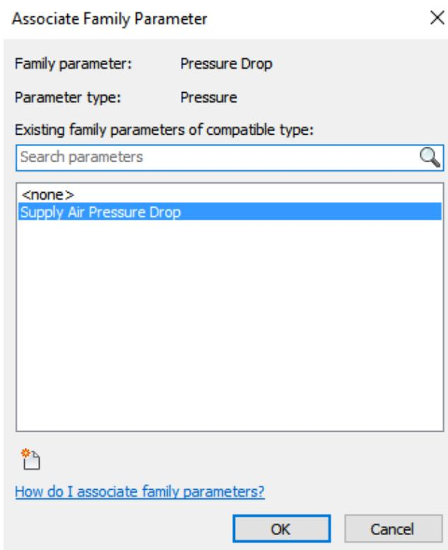
*Note: this value can be changed from "in-wg" to "PSI" or other format from the **Manage** tab, **Settings** panel, **Project Units** tool, and selecting the **HVAC** discipline, **Pressure value**:*
