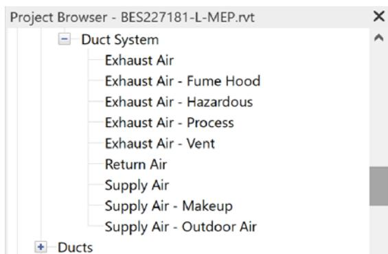
These are examples of **duct system types** that can be used in a project, and can be added to your project template using the **Transfer Project Standards** tool located on the **Manage** tab from this project when you get back to the office.
