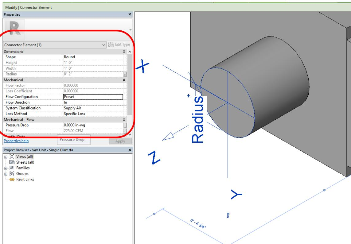
2. The connectors in this family are considered the **parent** connection in a system. **Flow configuration** determines how the flow is calculated, and **flow direction** is the data associated with the connector. For example, the airflow is considered *out* from the main air handler *in* to the VAV unit, so leave the direction set to **in**.
