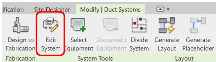
The source equipment can be selected at several different points, including the **Modify | Duct System** tab when the system is first defined, or after the initial system has been created.
