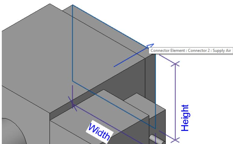
The two connectors are linked, and the round connector is defined as the **primary connector**. Information from this connector will pass to the outlet connector #2.
