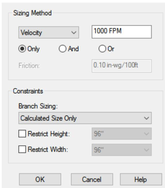
8. Make sure **Velocity** is set to **1000**. Change the **Sizing Method** to **Friction**, making sure the value is set to **0.12**, and then set the **Branch Sizing** to **Match Connector Size**:
