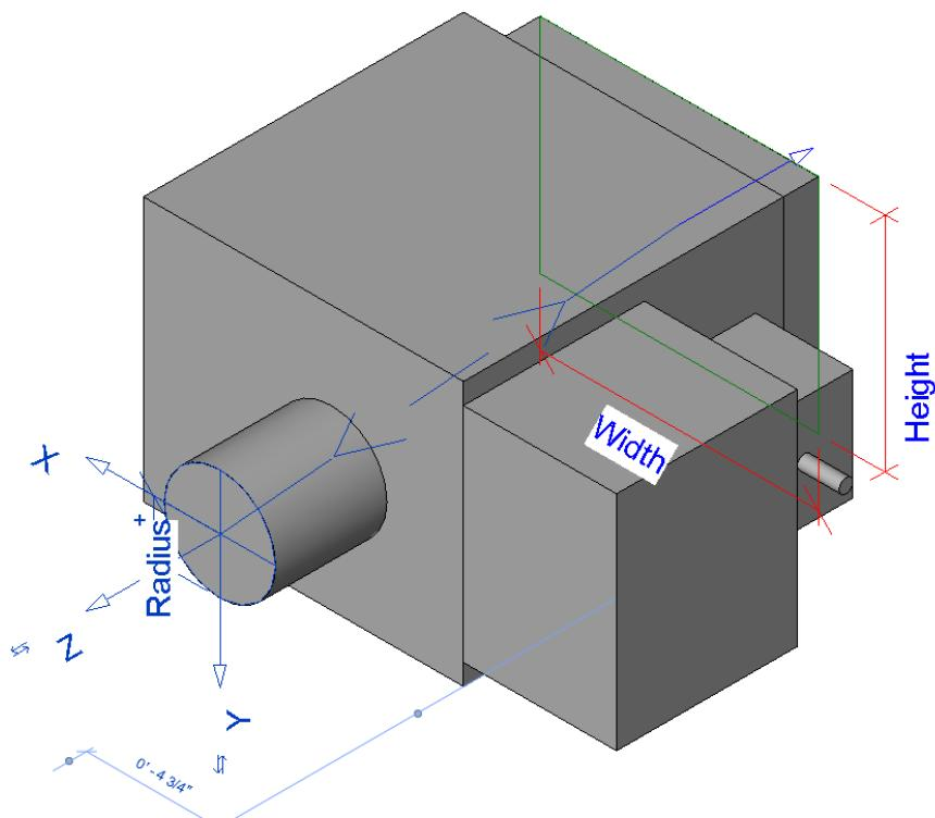
Once the link is removed, the total air flow and pressure drop on the rectangular connector will be based on the values assigned to the air terminals that make up the system. The properties assigned to the round connector, the inlet, will be used to define data as a target, and will be transmitted to the air handling unit servicing this unit.
