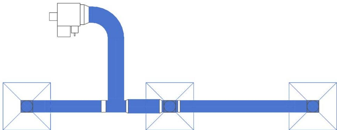
Note that there may wind up being a few pieces that don't size the exact direction you want – but these can be easily modified. Using the System Inspector in conjunction with the sizing tools can get you the best results.
