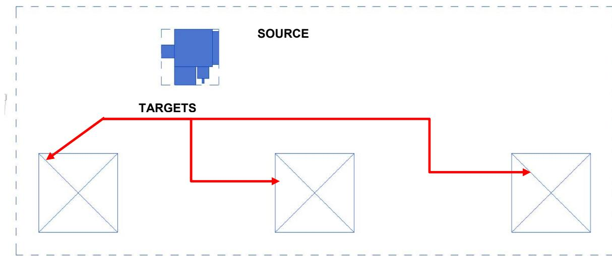
The system is now a well-formed system, and includes **targets** (the air terminals) and a **source** (the VAV unit).
