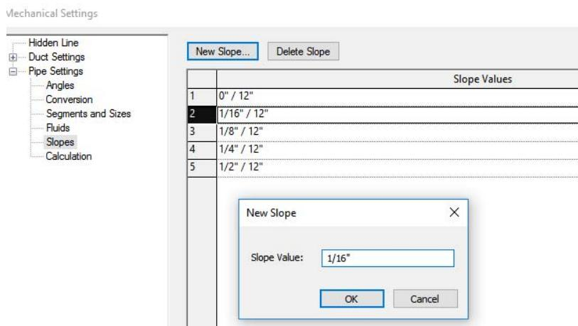
Click **New Slope** and then enter **1/16"**. The new size will automatically include the **run** value. The slope will be available when the pipe routing solutions are available.
