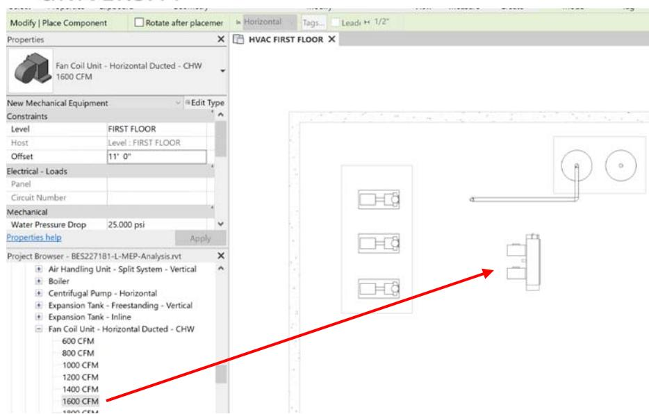
Place the unit 11' above the First Floor Level. Make sure the unit is rotated so the connections are pointing at the pipe.
