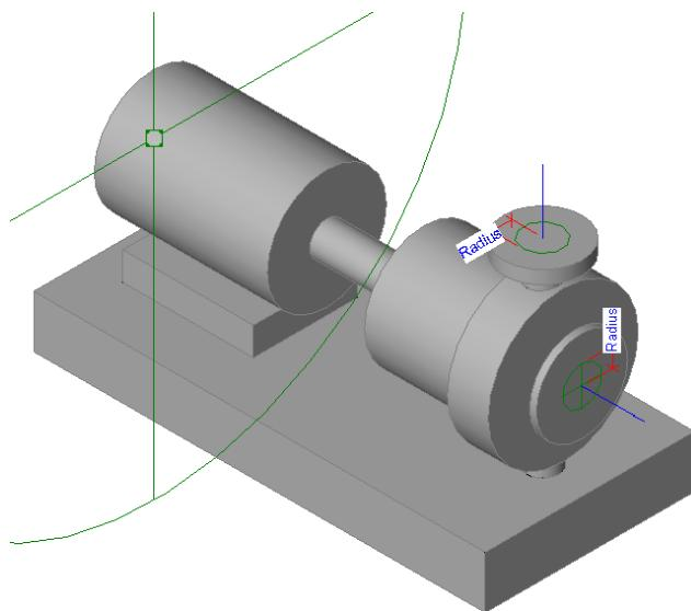
1. From the 3D view, rotate the view to show the **suction connector**. **Select the pipe connector element** and then **review the Properties**:
