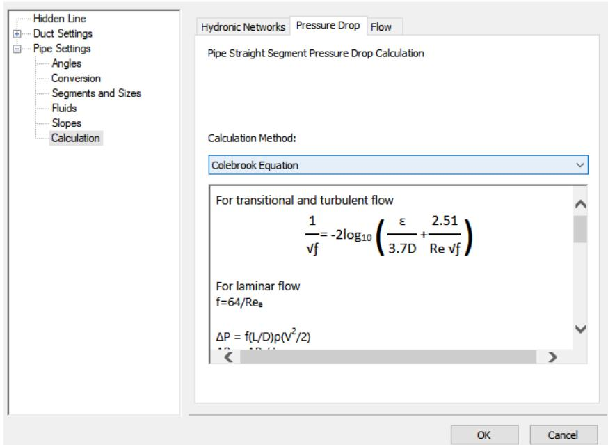
In earlier releases, you could only use the built in formulas while making minor modifications in the pipe system. Now, you can choose between different methods and formulas to calculate pressure drop based on the *Colebrook*, *Haaland* and *Simplified Colebrook* equations.
