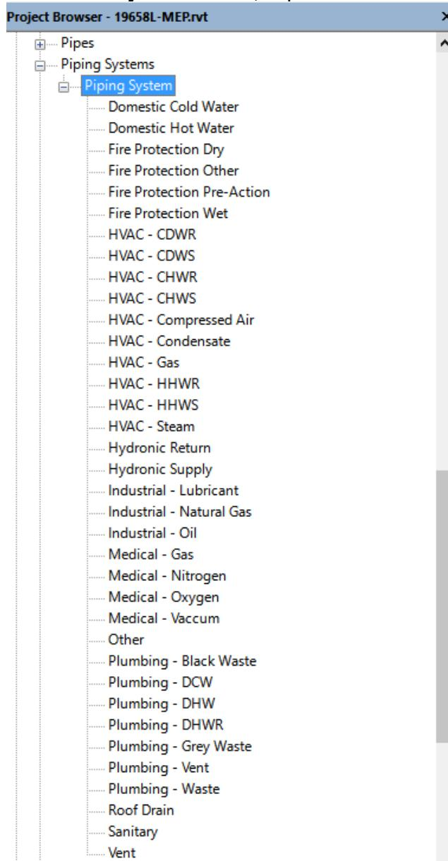
These are examples of **pipe system types** that can be used in a project, and can be added to your project template using the **Transfer Project Standards** tool located on the **Manage** tab from this project when you get back to the office.
