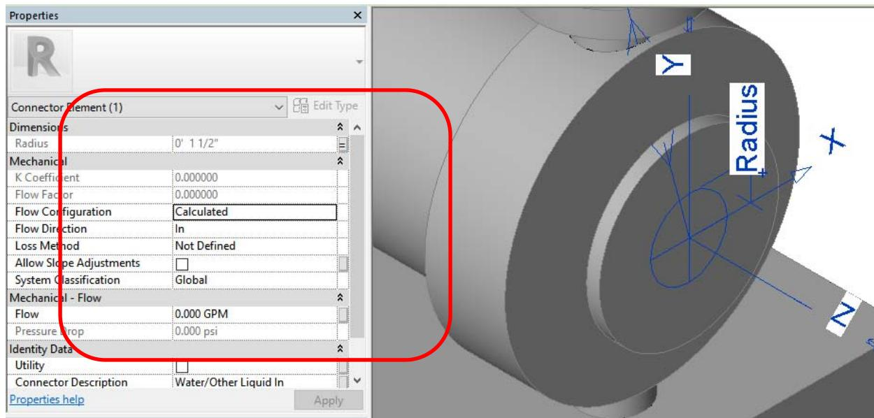
2. The connectors in this family are considered the **child** connection in a system, since the tank is the source (parent). But, a pump can be both a target and source, so it depends on how the connection is defined. If the pump was selected as the source in this system, then it would be considered the parent. Understanding this relationship is key to understand the role of the flow values.
