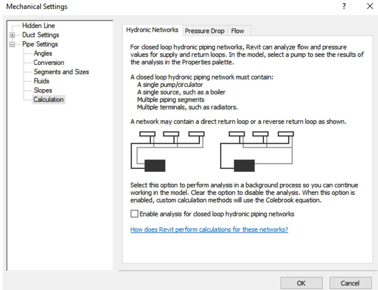
The settings allow you to set the calculation method for closed loop hydronic piping networks, for calculating pressure drop, and calculating flow based on fixture units for domestic water and sanitary systems.
