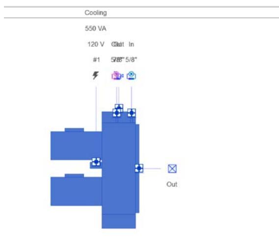
3. Next, **select the pipe where the connection should be made**. The pipe should be the same **system classification** as a pipe connector in the model – if there is more than one connection, the connection that matches the system classification for the pipe connector is used, and the connection is defined:
