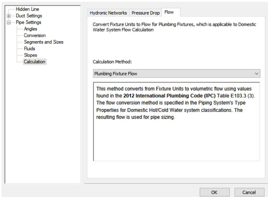
The **plumbing fixture flow** calculation method is based on the **2012 IPC table values**, and is the only method available.
