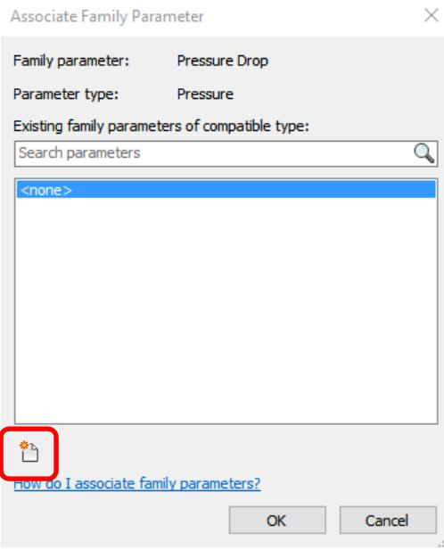
6. The Parameter Properties dialog appears. Normally you would use a shared parameter to control this data, if the information is intended to be included in a schedule. For this class, leave it as a family parameter, so it can still be exposed and edited in a project. **Name the new parameter Suction Pressure Drop, and leave all of the remaining settings as is:**
