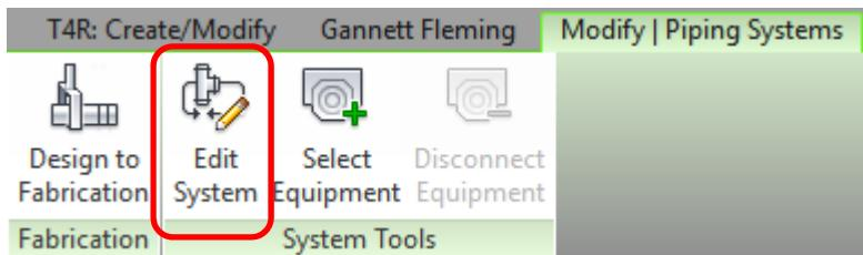
The source equipment can be selected at several different points, including the **Modify | Pipe System** tab when the system is first defined, or after the initial system has been created.
