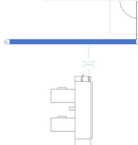
7. **Rotate the fan coil unit 90 degrees** – the connection will be maintained:
