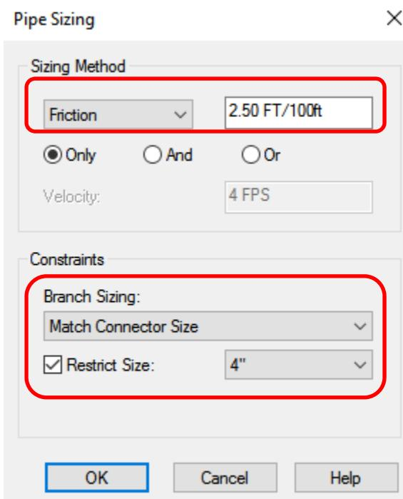
6. Click **OK**, and the pipe will be resized if needed. If the sizing fails, or nothing changes, check for an error message in the lower right corner:
