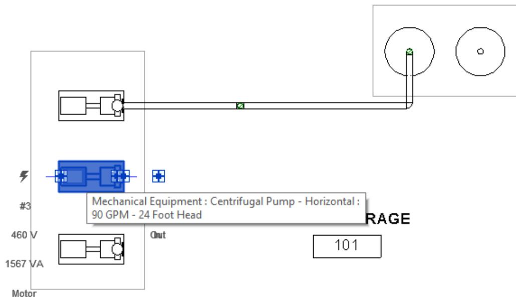
2. Once the pump is selected, [click Piping from the Modify | Mechanical Equipment tab](#):
