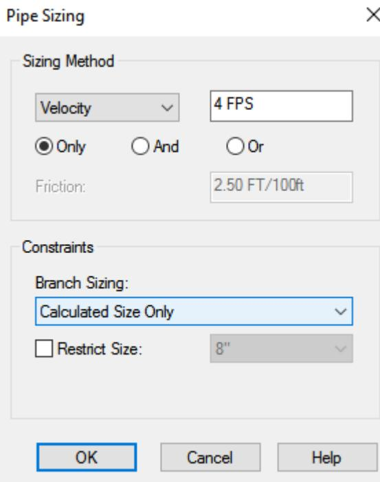
5. Change the **Sizing Method** to **Friction**, making sure the value is set to **2.5**; and then set the **Branch Sizing** to **Match Connector Size**; and then **Restrict the Size** to **4"**:
