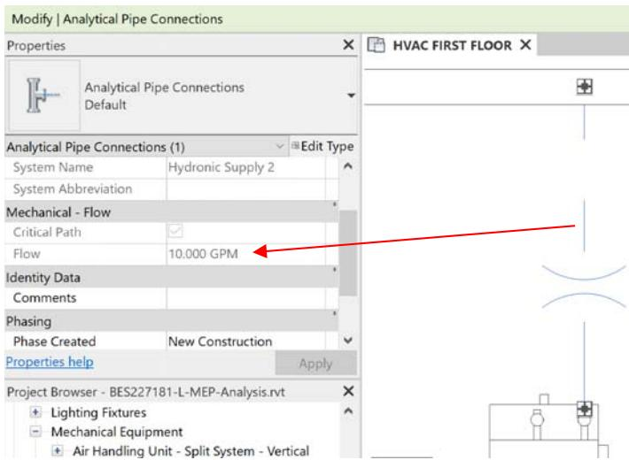
5. To change this value, select the equipment and review the **Chilled Water Flow** instance property. **Change the flow to 10 gpm**:
