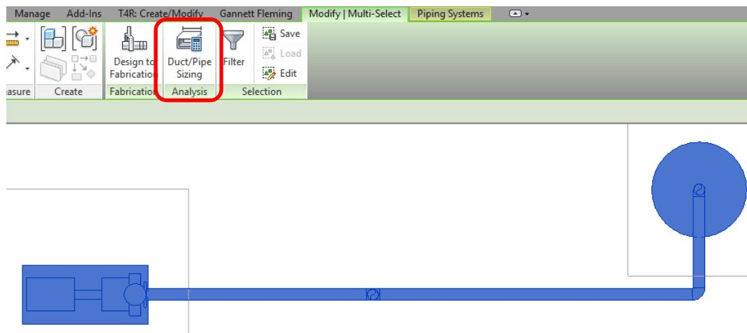
4. Select the **Pipe/Pipe Sizing** tool from the **Analysis** panel. The **Pipe Sizing** dialog will appear:
