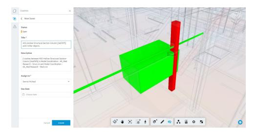
TIP: Critical elements intended for clashing are defined by what is visible in the published 3D view associated with the models loaded into the Coordination Space. Filter this content to remove unnecessary, erroneous clashes from oversaturating the clash results.
