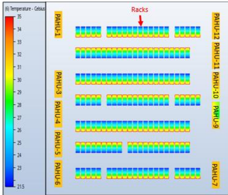
Temperature contour plot for servers at middle of server rack
