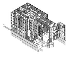
Revit model striped to necessary parts for simulation
