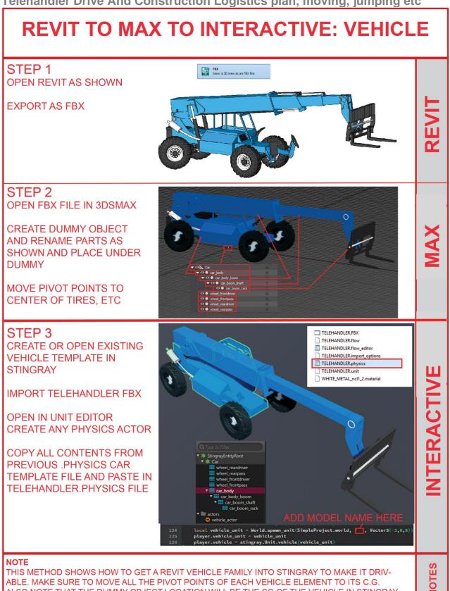
ALSO NOTE THAT THE DUMMY OBJECT LOCATION WILL BE THE CG OF THE VEHICLE IN STINGRAY
