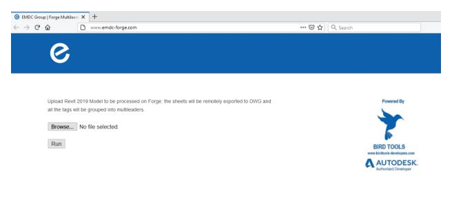
Whenever the Revit cloud add-in receives the corresponding request, it runs the scripts and generates the output files. The add-ins themselves, both the Revit and AutoCAD ones, are DLL Class libraries compiled to operate on top of the .NET environment. These classes can be written
