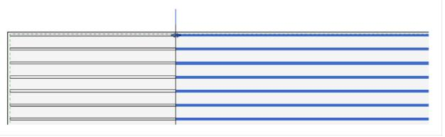
• **Split at Element** – This is a new feature, dedicated to split rebar distribution by selecting a structural element which will be the dividing element. In the following example, a beam was selected to cut all longitudinal rebars.
