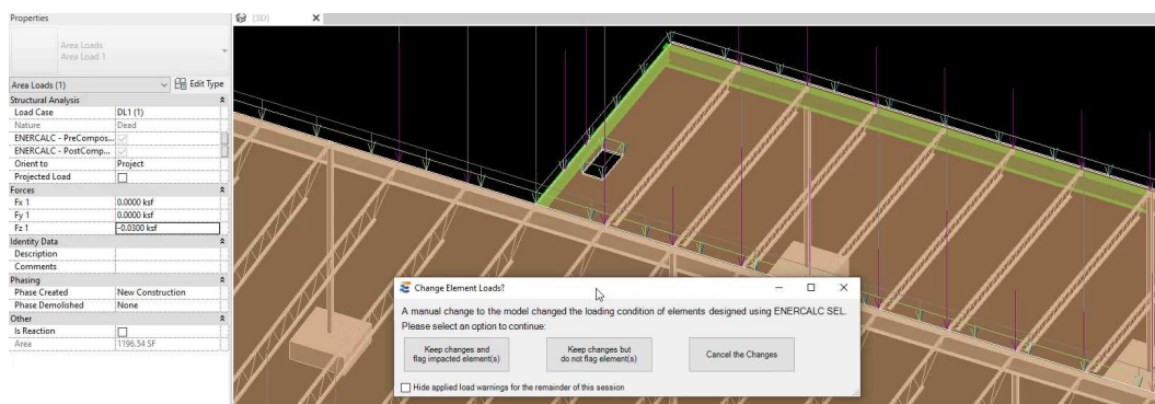
FIGURE 33: MODEL CHANGE NOTIFICATION TRIGGERED BY AREA LOAD CHANGE
