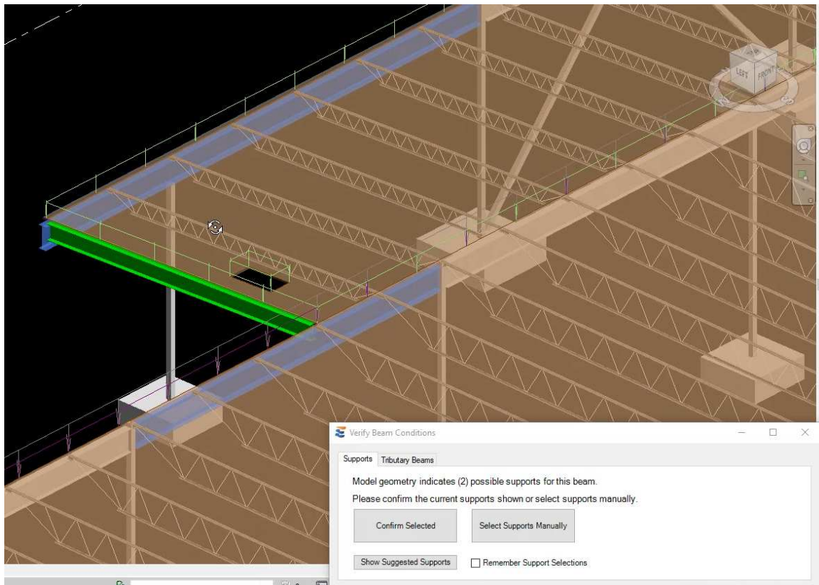
FIGURE 24: LAUNCHING EDGE BEAM WITH ADJACENT DECK OPENING
