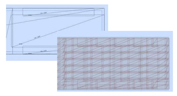
For the foundation beams we used similar method as with the frames where we change the slabs to claddings and could receive the linear loads which is distributed to the beams. In that way, we could perform a reinforcement calculation, unfortunately this part was done manually after we received the right linear loads.
