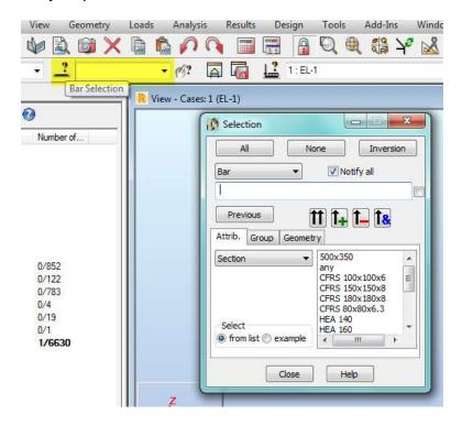
When we later have completed the model check we can start the calculation part of the static forces. I will highly recommend that we start by doing a quick calculation with just a dead load to assure that we do not get warnings that will be critical for the results. If that step is ok then we can proceed with the correct load-cases and combination.
