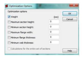
At last we could finally press calculations button to get an overview of the verification. All the objects that had an utilization of more than 100 % were increased in section and those with low utilization was decreased, because of esthetic part was a thing we wanted to maintain we instead used the same type section for the certain frame, we didn't want to have different size of the section on the same frame.
