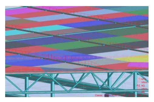
The next step will allow us to examine the results such as moments, normal-/shearforces and reaction forces which will define the loads the piles will carry.
