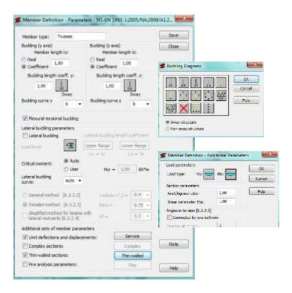
To be able to have more control of the objects we decided to divide the objects into groups for the optimization. We had specific groups for columns, one for trusses and another one for the beams. The optimization is a process which is performed in several iterations to finalize a complete utilization of the objects.
