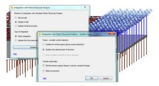
Export steps when we have added objects in Robot that needs to be transferred to Revit.
