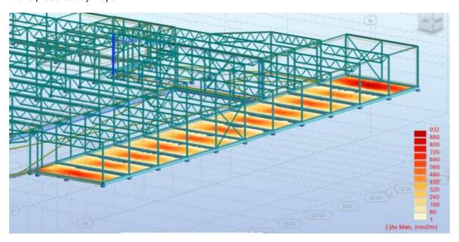
After we received the required reinforcement we could easily go further to Provided Reinforcement and define which fabric area we wished for and apply it to the plate.
