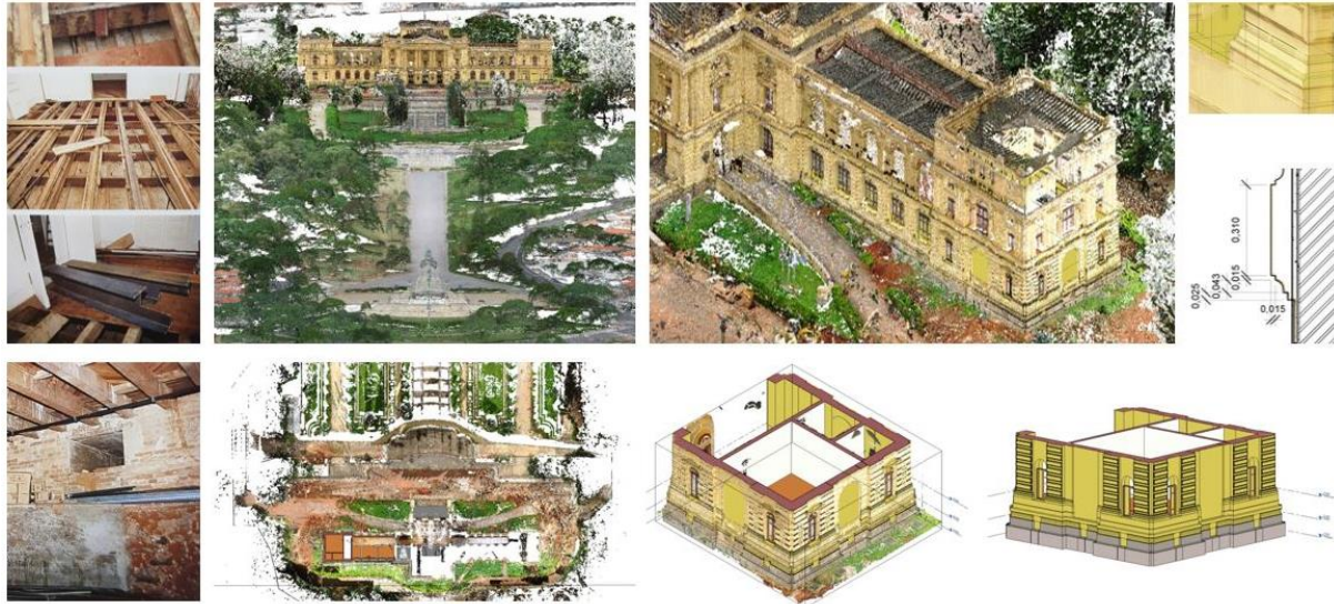
Figure 10 – Scan-to-BIM process in Revit.
