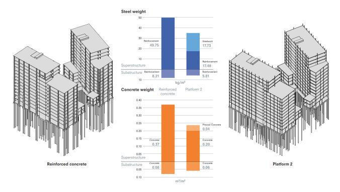
Relative weight of material - Platform vs. traditional construction
