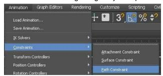
to the second stop for 5 seconds, repeat the 2 second pause, then travel to the end point over the next 6 seconds. So we'll start by assigning a Path Constraint to each point helper and link it to its corresponding spline. Next, move the keys that were generated to set the timing of the motion as indicated above (Point01 start 0, end 150; Point02 start 210, end 360; Point03 start 420, end 600).
