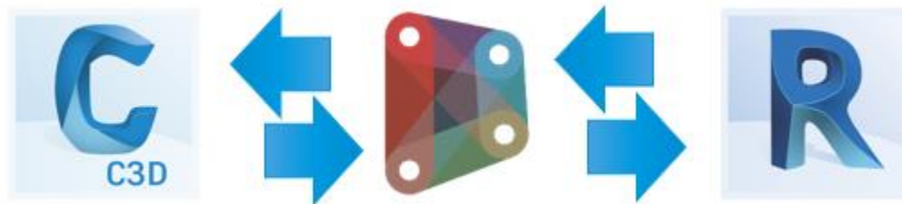
FIGURE 9: CIVILCONNECTION & CIVILPYTHON DYNAMICALLY CONNECT CIVIL 3D AND REVIT VIA DYNAMO
