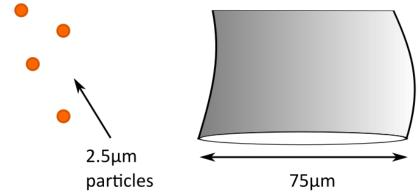
$PM_{2.5}$  PARTICLES ARE SHOWN HERE IN COMPARISON TO THE DIAMETER OF A HUMAN HAIR
