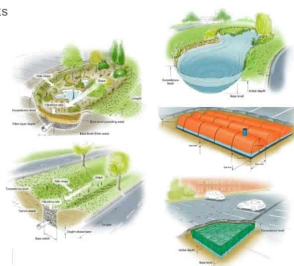
Storage Structures and Green Infrastructure are represented by feature lines connected by a mesh surface. The feature lines can be edited for round tripping both in terms of changing shape and levels.
