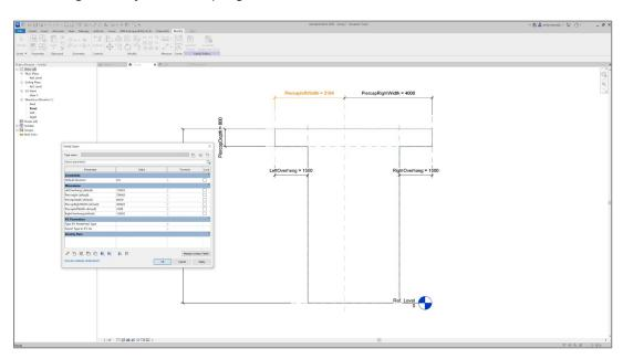
We can then switch to the reference level to repeat the above steps to define the thickness of the pier.
