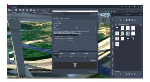
The existing pier can then be selected and changed to the newly created component and configured in the panel to suit.
