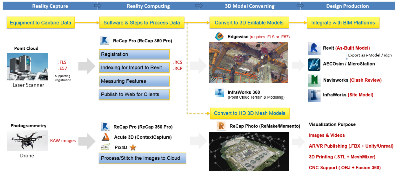
FIGURE 5: SHOWS THE TOOLS AND PROCESS DURING EACH PHASE OF SCAN TO BIM JOB
