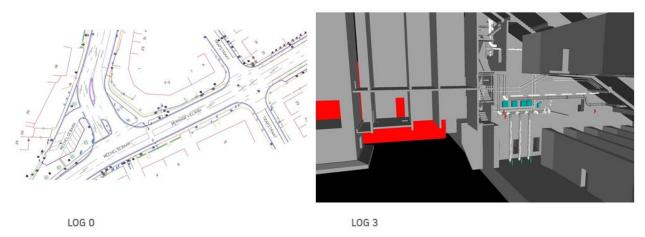
FIGURE 6: EXAMPLES OF DIFFERENT LEVELS OF GEOMETRY (LOG)
