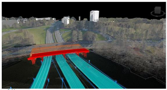
FIGURE 5: MODEL OF EXISTING AND NEWLY DESIGNED INFRASTRUCTURE COMBINED WITH AVAILABLE PUBLIC DATA SOURCES FROM THE INFORMATIE VLAANDEREN AGENCY
