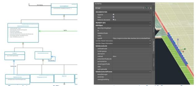
FIGURE 3: IMPLEMENTING OTL INFORMATION REQUIREMENTS (DIAGRAM LEFT) IN CIVIL3D PROPERTY SETS
