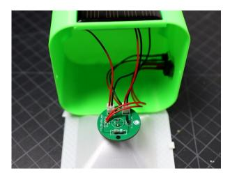
At last install the PCB on the front reflector. Use hot glue to fix all the components with the 3D printed enclosure.
