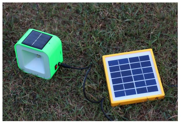
To test the lamp, cover the solar panel by your palm, the LED should glow. If the LED light up, then the circuit is working perfectly.
