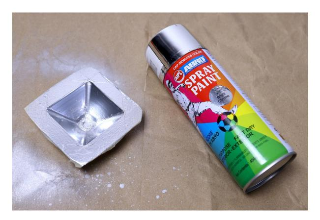
Before applying the paint, cover the edges of the enclosure with a masking tape, so that paint will be only applied on the reflector part.
