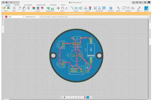
Arrange all the components in such a way that the board occupies minimum space. The smaller the board size, the cheaper will be the PCB manufacturing cost. It will be useful if this board has some mounting holes on it so that it can be mounted in an enclosure.
