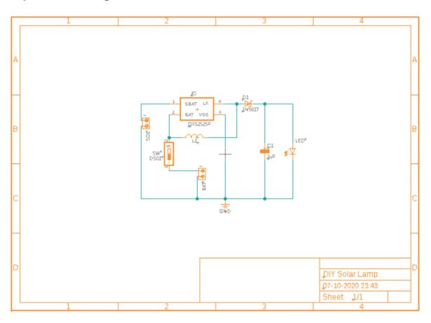
I have drawn the schematic by using Fusion 360 Electronics Design after that switched to PCB layout. All of the components you added in the schematic should be there, stacked on top of each other, ready to be placed and routed. Drag the components by grabbing on its pads. Then place it inside board outline.
