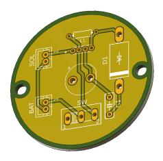
Now you have to route. Routing is the most fun part of this entire process. It's like solving a puzzle! Using the route tool we need to connect all the components. You can use both the top and the bottom layer for avoiding overlap between two different tracks and making the tracks shorter. In the end, using the polygon tool, we need to create the ground area of the PCB.
