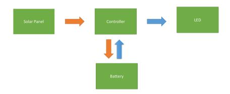
The solar lamp is a standalone SPV system and contains four components of Standalone SPV system:
