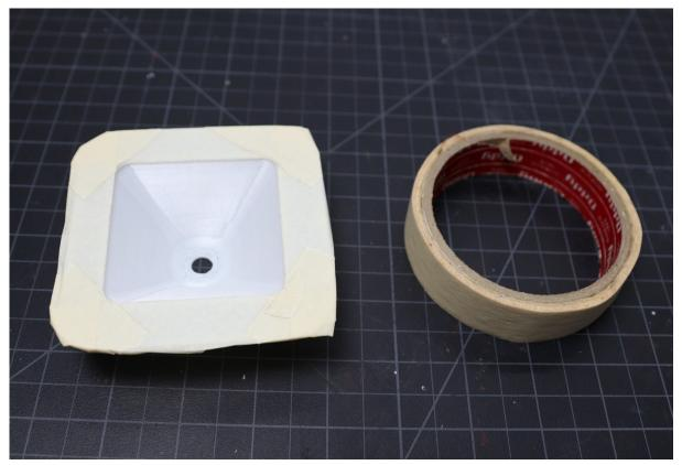
The reflector can be purchased directly from the market, but to reduce the cost, it is considered to be a part of the 3D printed enclosure. Only you have to apply few coats of reflective spray-paint on the 3d printed reflector. Here I have used bright chrome spray paint, it works really nice.
