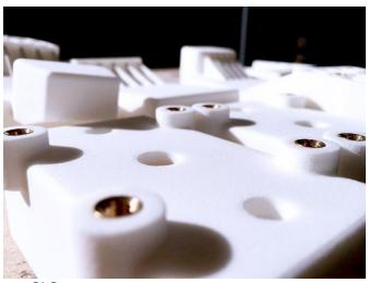
SLS NYLON PARTS WITH INSTALLED BRASS INSERTS
