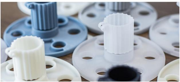
SLA PARTS HAVE SMOOTH SURFACE FINISHES AND HAVE AVARIETY OF RESINS WITH DIFFERENT PROPERTIES
