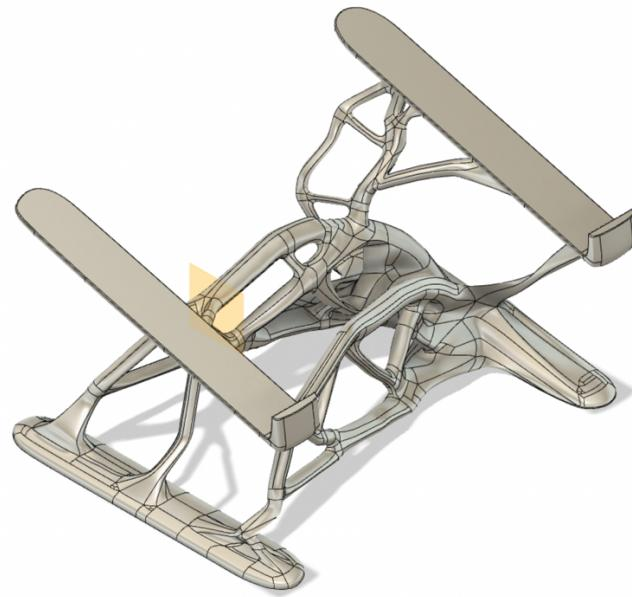
A quick form study using T-Splines geometry shows a more practical direction, where the GD frame can be used on the side ends only.
