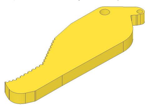
The starting shape is the initial shape from which the solver generates the outcome. The starting shape is optional.
