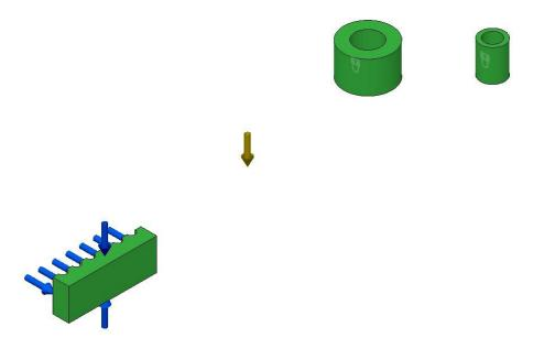
The preserve geometry typically includes the connection points to attach the design to other objects or interact with them or you interact with, such as handles. This is the geometry where you apply the loads and constraints for the study. This geometry is incorporated into the final design.
