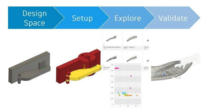
For completing the set up, the Design Conditions (Loads and Constraints), the Design Criteria (Optimization objectives and Manufacturing constraints) and the materials must be defined.
