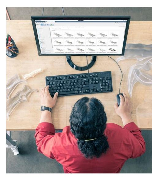
Designers or engineers input design parameters (such as materials, size, weight, strength, manufacturing methods, and cost constraints) into generative design software and the software explores all the possible combinations of a solution, quickly generating hundreds or even thousands of design options. From there, the designers or engineers can filter and select the outcomes to best meet their needs.
