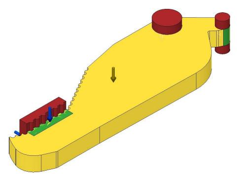
The first step for setting up a Generative Design study consists in creating the geometries of the Design Space. That is, the preserve geometry, the obstacle geometry and the starting shape (optional)
