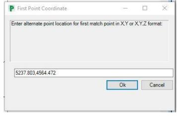
d. If the points you chose match in distance, no errors will be received, and you will get a dialog box allowing you to name this new coordinate system. However, if the points chosen do not match in distance, APL will display a message showing the difference. In the example shown here, 0.18 feet is approximately 2-1/8"
