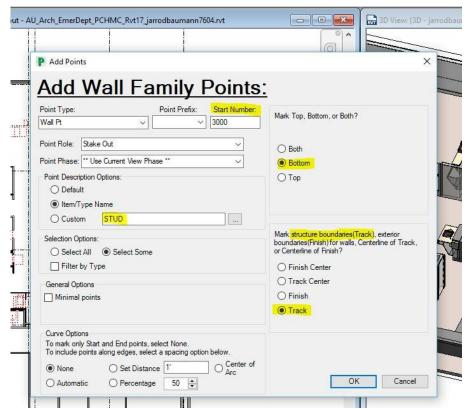
2. Using a floor plan or 3d view, you can immediately begin selecting walls to add our layout points to. When finished adding walls, choose Finish from the options menu. APL will points to all selected walls.
