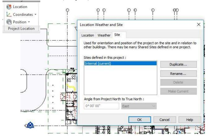
Here we can manage and setup multiple coordinate systems within the same Revit model. For example, we may use one coordinate system as the origin for our internal MEP BIM coordination process and another to orientate our building to a geospatial location such as the horizontal control typically found on the civil contract drawings.
