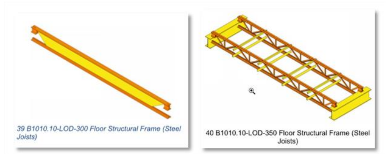
LOD 300 vs LOD 350 for steel joists
