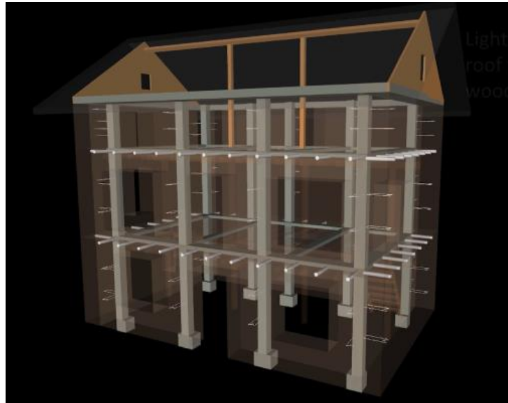
A specific type design used in Nepal, featuring strongbacks (columns) connected to a ring beam on top of the walls and a lightweight roof.
