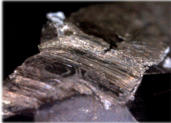
Figure 10 - The cutting edge of a Z-Carb tool after it has been used to cut Inconel-718 with steel settings
