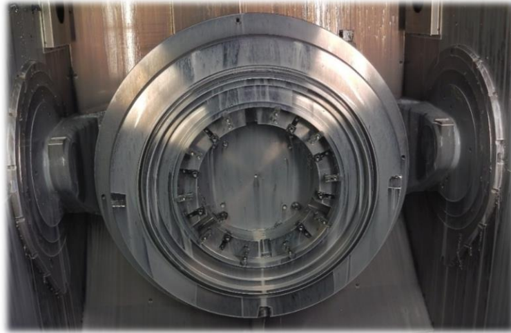
Figure 26 - An image of slots being cut into the outside of the blisk in such a way as to regulate hoop stress
