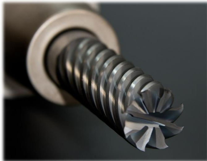
Figure 1 - An image of an end mill showing eight cutting edges and flutes (Schwarzenberger, 2014)
